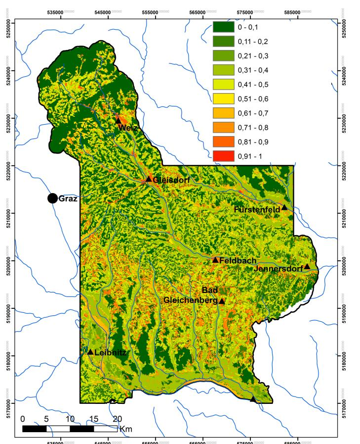
Runoff coefficients were modeled using the HYDROBOD model (see Klebinder et al. 2017 for references). The model calculates runoff for various layers (infiltration, soil, and geology), for instance, surface runoff coefficients for a rain event (1 h, 64 mm) in the above map.
