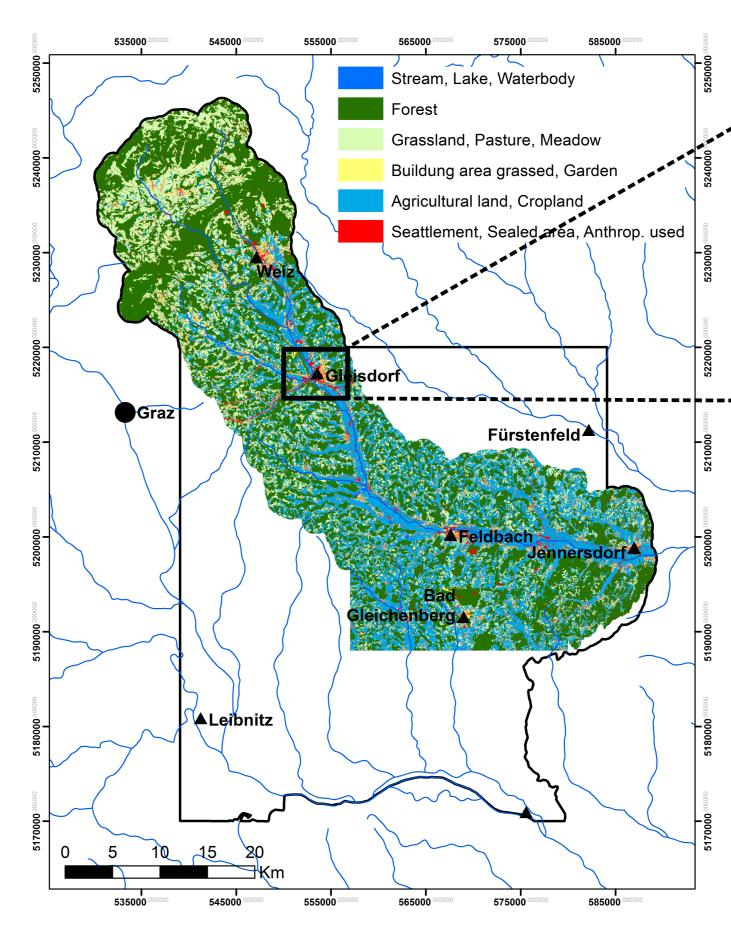
Detailed land use / land cover data were generated using a digital cadaster map, data from the Austrian forest map, from the EU's Integrated Admission and Control System (IACS/INVEKOS) and from orthophotos. The resulting map shows clear improvements over the widely used CORINE data.
